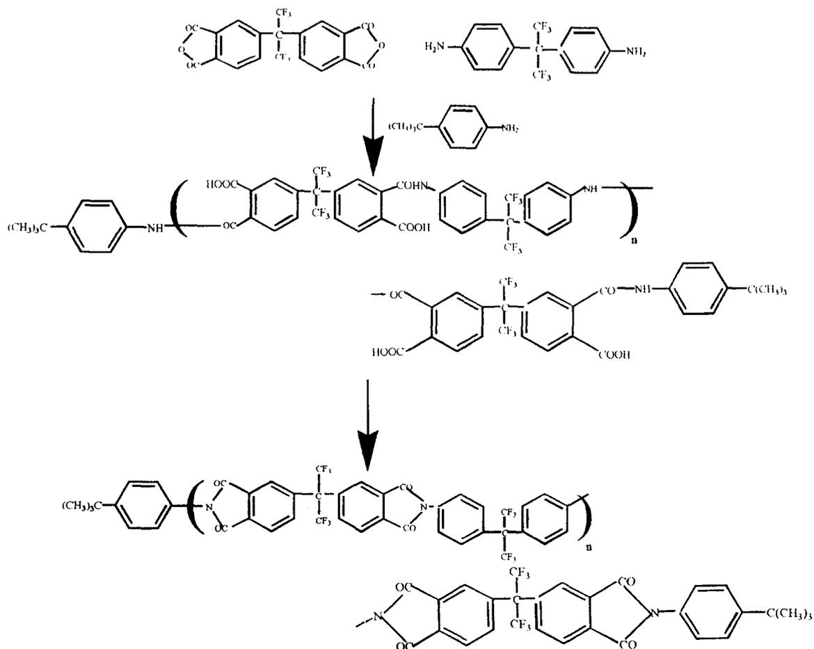
Figure 2 Preparation of 4-tert-butylamine-terminated polyimide based on 6FDA and 6FDAM with controlled molecular weight
