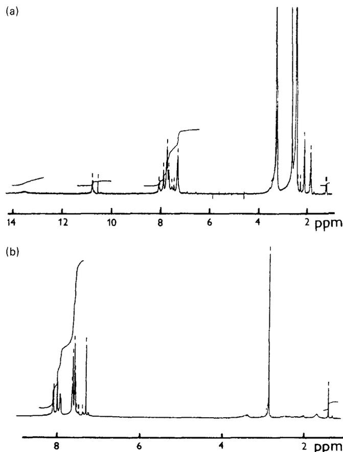
**Figure 3** <sup>1</sup>H n.m.r. spectra of 4-*tert*-butylaniline-terminated PAA (a) and PI (b) based on 6FDA and 6FDAM with controlled molecular weight
